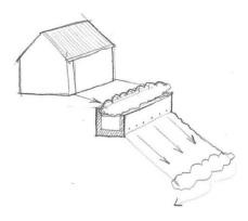
Flow-through planter built into a hillside. Flows from the underdrain and overflow must be directed in accordance with local requirements.
