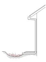
Connecting a roof leader to a vegetated area. The head from the eave height makes it possible to route roof drainage some distance away from the building.
