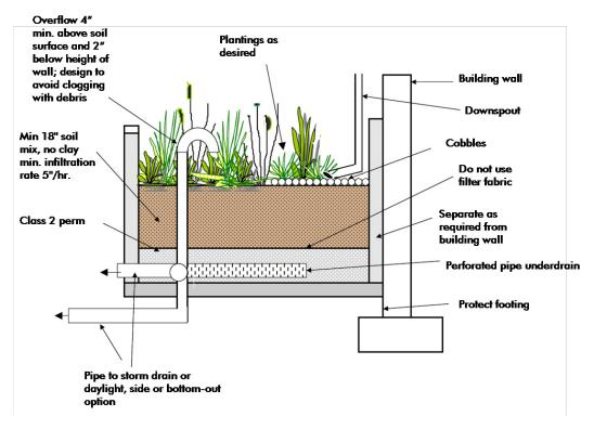
Planter boxes can be constructed adjacent to buildings or set into slopes. They are most effective when openbottomed, but can also be built to eliminate seepage to native soils if necessary to protect foundations or slopes.
