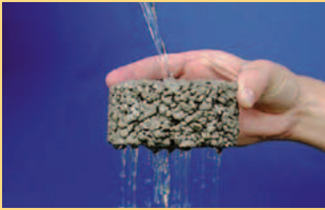
Pervious concrete allows rain to soak into the underlying soil.
