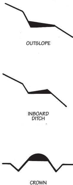
Types of surface road erosion
